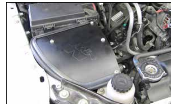
22. Install the K&N® filter lid and secure with the provided hardware.
