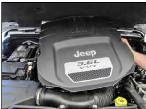
2. Lift up and remove the engine cover.
