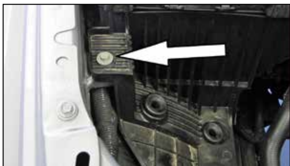
9. Remove the bolt shown that secures the air box mount bracket to the inner fender.
