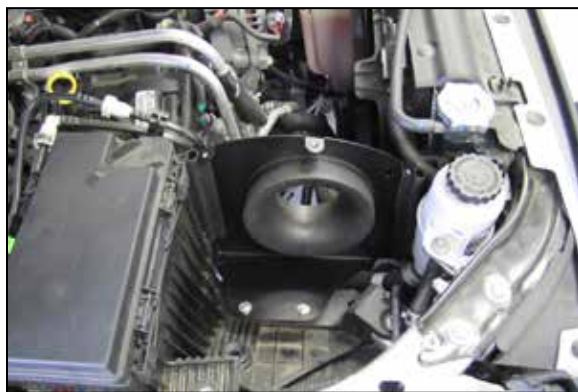
16. Install the heat shield assembly into position so the mounting studs are in the air box mounting grommets.
