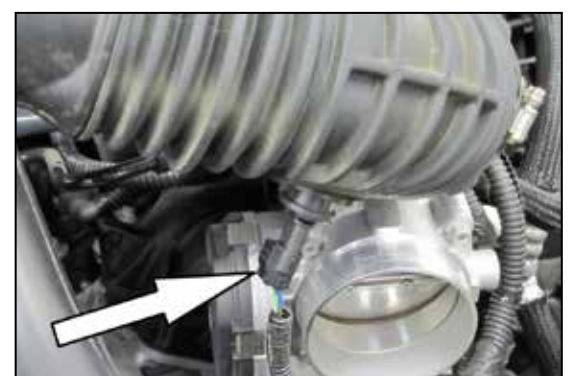
6. Lift up the intake tube and then disconnect the inlet air temperature electrical connection. Then remove the intake tube from the vehicle.
