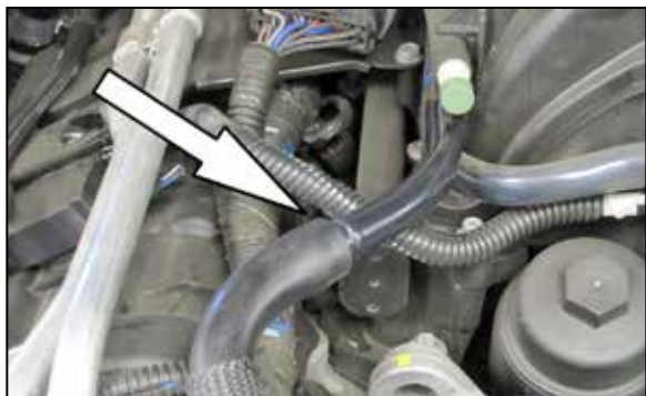
7. Disconnect the crank case vent hose from the crank case vent tube.
