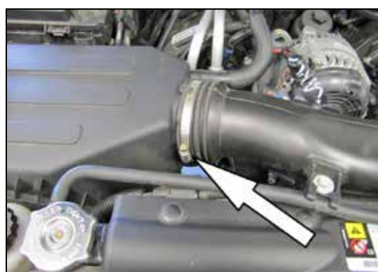
4. Loosen the hose clamp securing the factory intake tube to the air filter housing.
