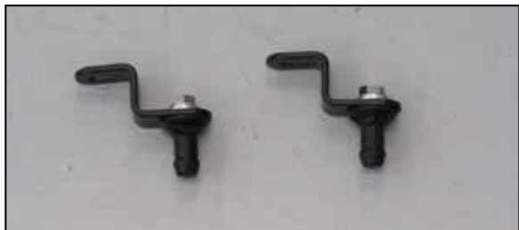
11. Install the two provided mounting studs onto the two heat shield brackets (070061) as shown.
