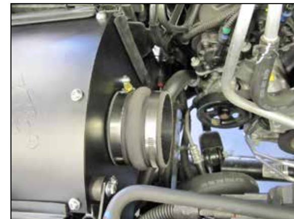
23. Install the provided hump hose (08699) onto the filter adapter and secure with the provided hose clamp.
