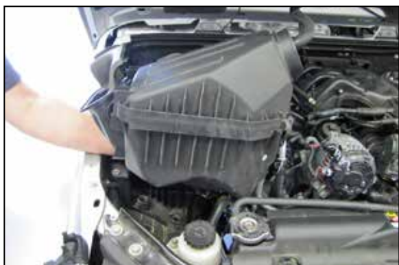
8. Lift up and remove the air filter housing from the vehicle
