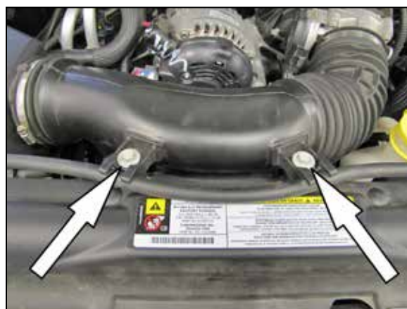
3. Remove the two bolts which secure the factory intake tube to the fan shroud.
