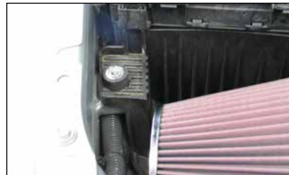
20. Install the rubber mounted stud into the into the air box mounting plate bolt location as shown.
