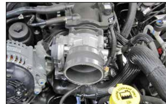
24. Install the provided silicone hose (08690) onto the throttle body and secure with the provided hose clamp.
